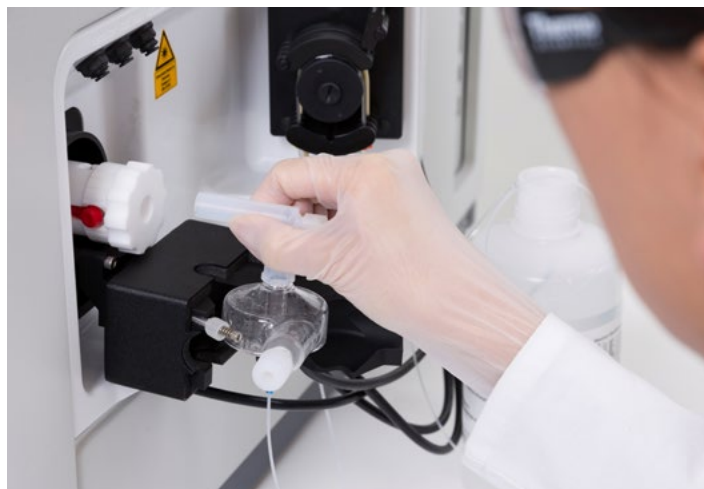
Figure 6.6 The small volume cyclonic spray chamber of the iCAP RQ ICP-MS allows fast wash out and reduced memory effects. It is push-fit connected to the torch assembly using a Teflon™ elbow connector and is housed inside a Peltier cooler for temperature stability, solvent removal, and reduction of oxides.
