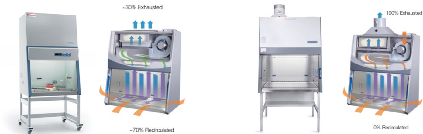
Figure 2.20 Flow of air within the A2 (left) and B2 (right) BSCs; most of the total air flow in an A2 gets recirculated back to the cabinet while 100% of the air flow in a B2 gets exhausted.
