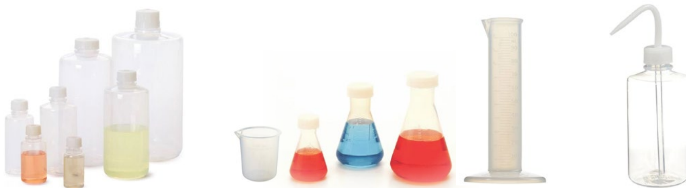
Figure 2.9 Various fluoropolymer laboratory apparatus: FEP bottles (left); PFA beaker, Erlenmeyer flasks, and graduated cylinder (center); and Teflon™ top dispensing wash bottle (right).
