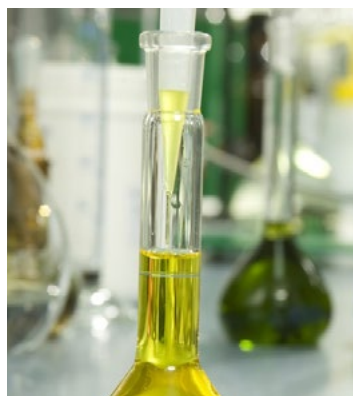
Figure 4.10 Pipette dispensing liquid into a flask with the tip in the center of the neck of the flask.
