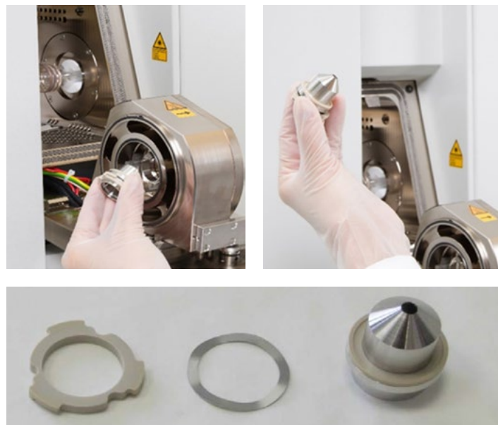
Figure 6.15 The extraction lens is located behind the drop-down door, bayonet mounted for easy removal.
