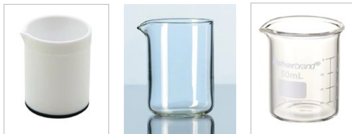
Figure 5.7 Griffin beakers made from different materials. PTFE (left) is best for ultra-trace detection limits, high purity quartz (center) is a better alternative to borosilicate glass (right). Borosilicate glass is suitable for higher detection limit applications or general laboratory work.
