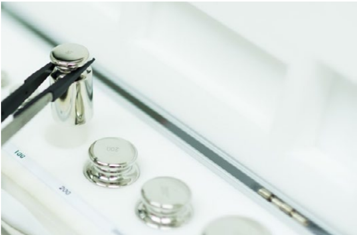
Figure 2.14 Documented periodic or daily inspections of analytical balances using certified test weights is a way to ensure the accuracy of weights measured.
