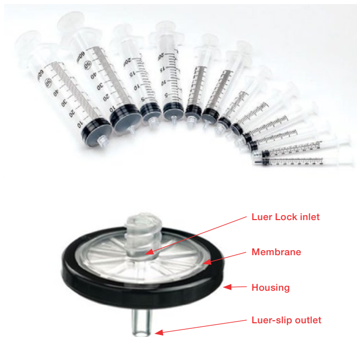
Figure 5.8 Disposable plastic syringes and syringe filters are recommended for filtration of samples prior to ICP-MS analysis. Pictured are Luer lock syringes (top) and a PTFE syringe filter (bottom).
