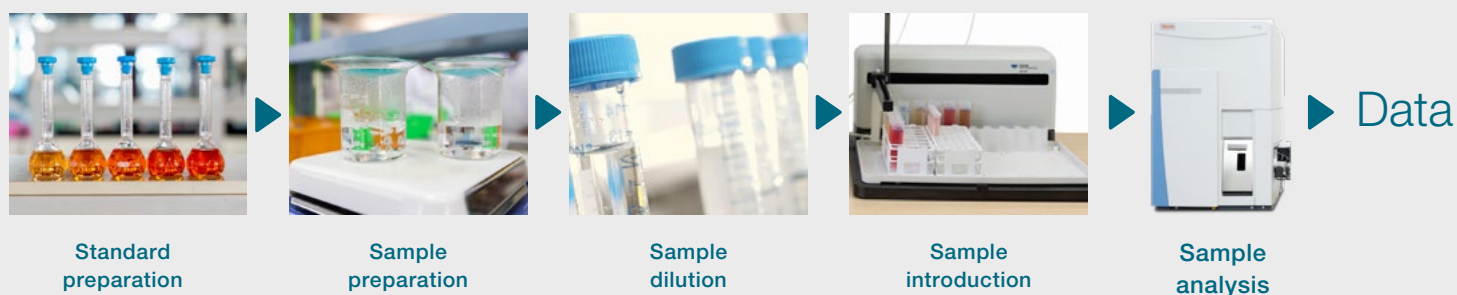
Figure 2.1 Processes within a typical element analysis workflow.
