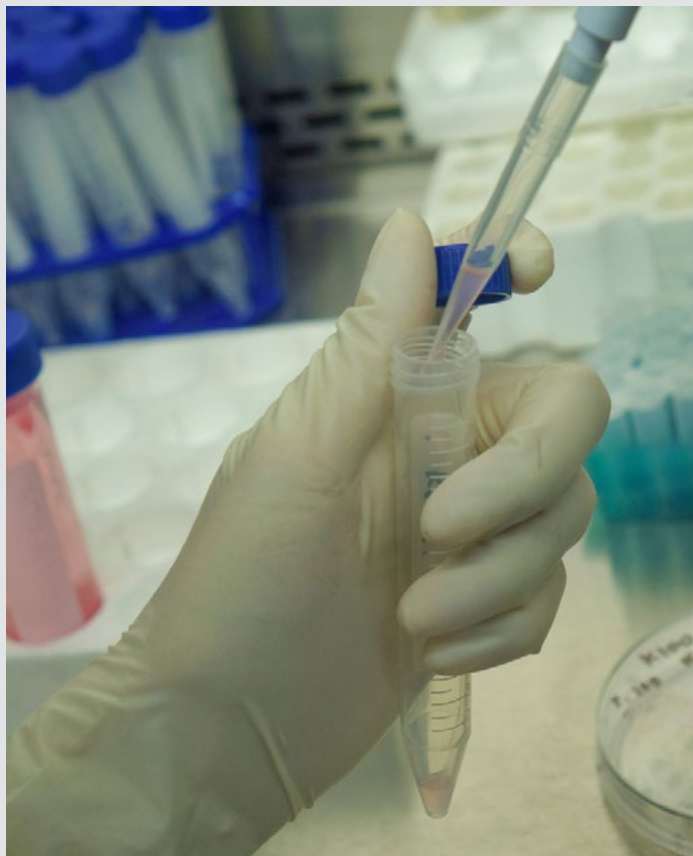
Figure 4.2 When filling an autosampler tube with a standard, it is best practice to use a calibrated and inspected mechanical pipette.
