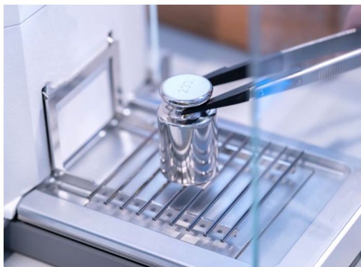
Figure 4.6 Analytical balances should be spot checked prior to use when preparing standard solutions.
