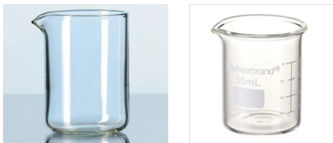
Figure 2.7 Quartz beaker (left) and borosilicate glass beaker (right). Quartz beakers, and other quartz apparatus, typically do not have graduated markings.
