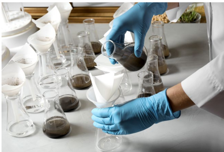
Figure 5.9 Traditional method of filtering samples involves pouring samples into a funnel lined with filter paper and collecting the filtered sample into an Erlenmeyer flask (left) or beaker (right).
