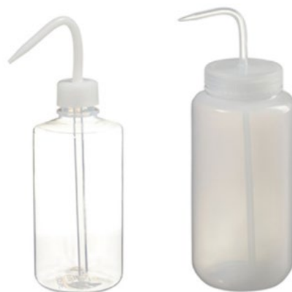
Figure 4.8 For ultra-trace analysis, Teflon™ (left) wash bottles are recommended for storing and dispensing acid diluents used to prepare standard solutions. For general purpose work or higher detection limit analyses, LDPE wash bottles (right) are appropriate.
