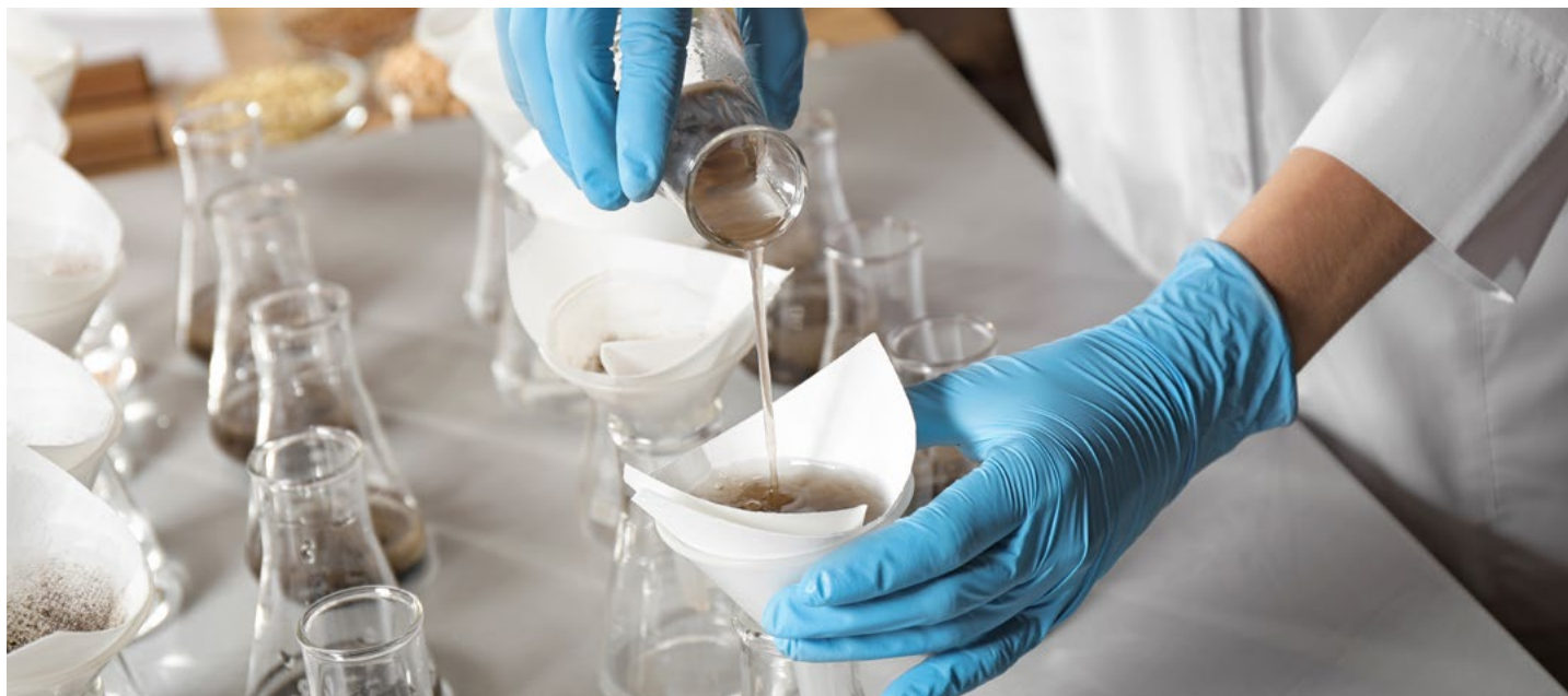
Figure 5.2 Sample solution after partial digestion containing suspended solids needs to be filtered prior to analysis.
