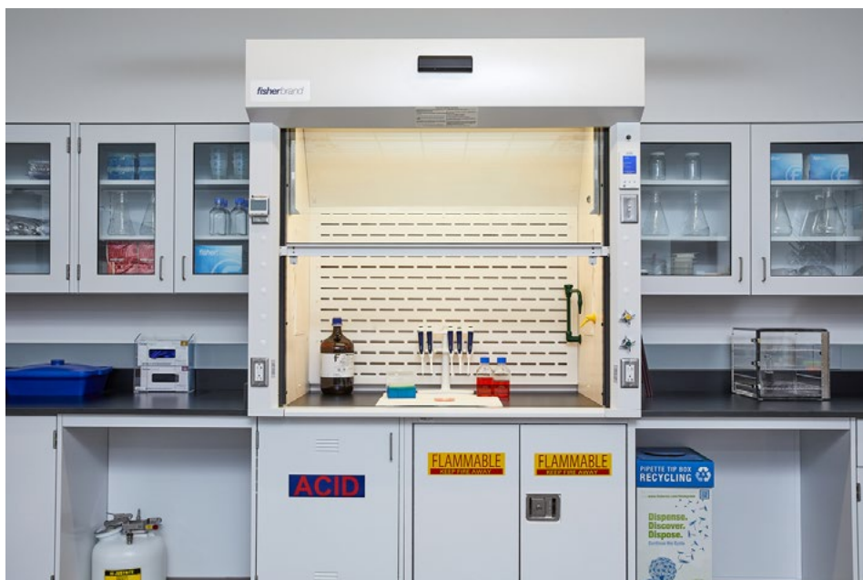
Figure 4.7 Preparations involving concentrated acids and other hazardous reagents must be done in a fume hood to protect the analyst and laboratory environment.
