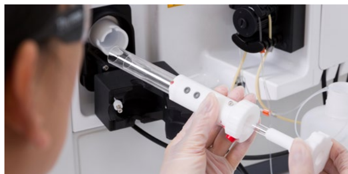
Figure 6.4 The streamlined design of the torch assembly allows fast and easy connection between components and installation to the instrument; no extra parts or tools required.
