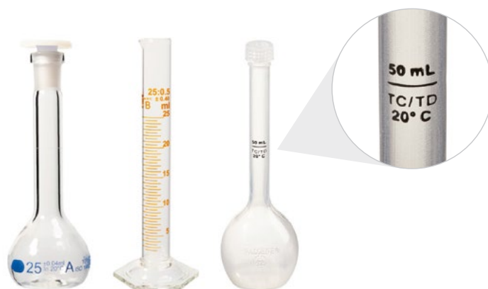
Figure 2.6 Laboratory apparatus with associated markings for Class A and Class B. On the right, a volumetric flask with markings designating both To Contain and To Deliver .
