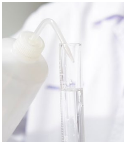
Figure 4.9 The addition of acid diluent using a wash bottle, wetting the walls of a container (left). Acid diluent should be filled to approximately half the volume of the flask prior to adding the stock standard to prevent analytes from adhering to the wall of the flask (right).
