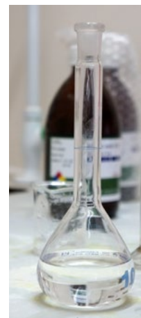
Figure 4.9 The addition of acid diluent using a wash bottle, wetting the walls of a container (left). Acid diluent should be filled to approximately half the volume of the flask prior to adding the stock standard to prevent analytes from adhering to the wall of the flask (right).
