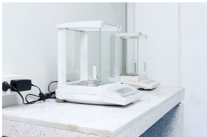
Figure 2.15 Storing analytical balances in the corner of a room away from sources of vibration, movement, direct sunlight, and ventilation help to ensure accurate measurements.
