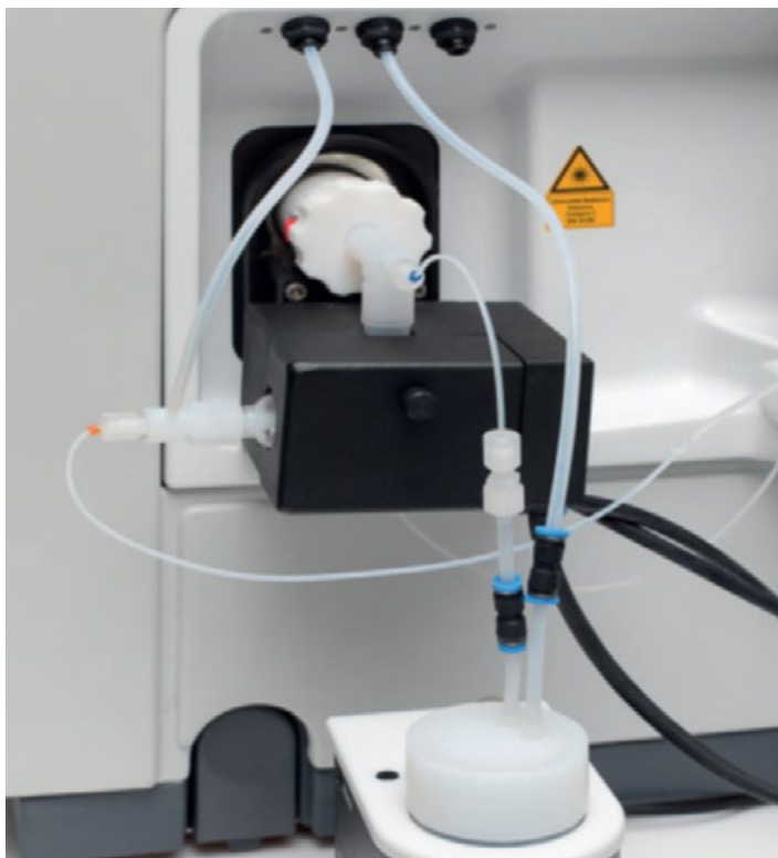
Figure 6.9 The Argon Gas Dilution set-up on the iCAP RQ ICP-MS. In this set-up, an argon humidifier is used to humidify an additional supply of argon added to the sample aerosol.
