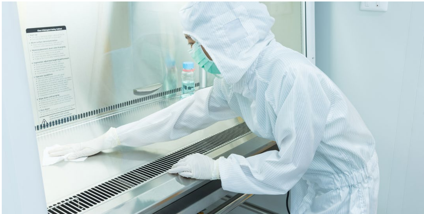
Figure 4.3 The work surface of laminar flow hoods should be cleaned prior to and after use.
