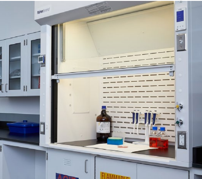
Figure 2.18 Fume hoods provide a safe, contained space for preparing solutions with concentrated, corrosive acids and other toxic chemicals. Always keep the fume hood workspace clean, clear, and organized when working with hazardous reagents.
