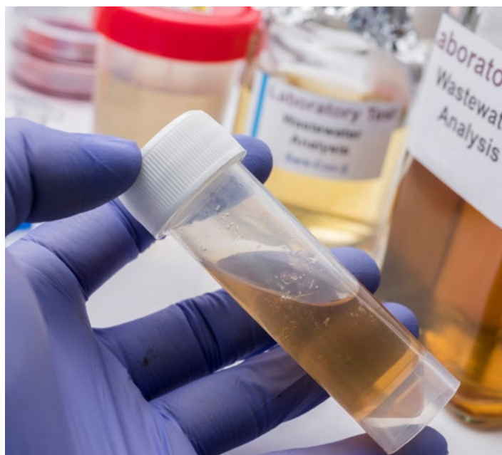
Figure 5.1 Samples from wastewater treatment plants (above) that contain suspended solids, high TDS, and organic material (below) require acid digestion.
