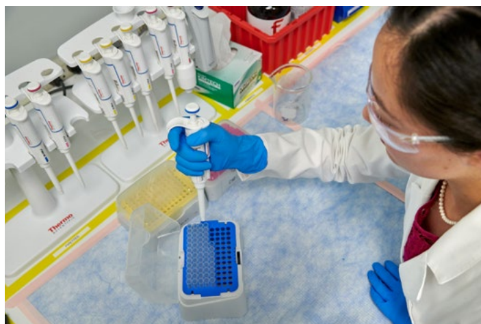
Figure 4.5 All necessary items for standard and sample preparation should be gathered and organized prior, including logbooks and forms to document preparations (top). Work surface should also be covered (bottom) to protect the surface and to prevent contamination from direct contact of apparatus to dust, dirt, etc., on the surface.
