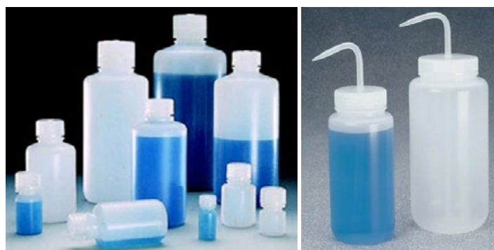
Figure 2.8 Various polyolefin plastic apparatus: (from top) PP graduated cylinders, container, holder, and LDPE unitary wash bottle; (bottom left) HDPE narrow mouth bottles; and (bottom right) LDPE top dispensing wash bottles.
