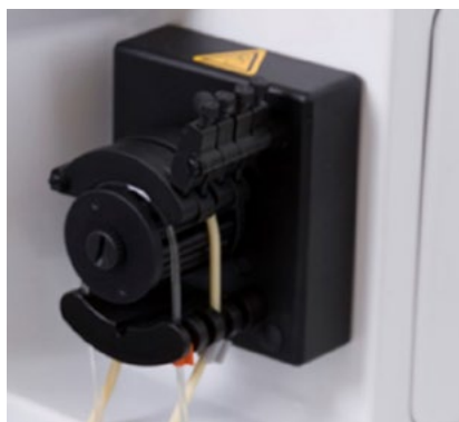
Figure 6.8 The sample introduction system and mini peristaltic pump of the iCAP RQ ICP-MS are located on the right side of the instrument at bench height. The mini pump has 12 rollers, 4 channels and inert rollers.
