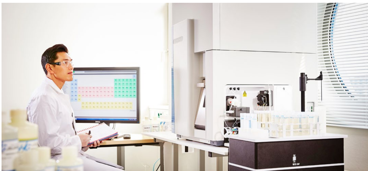
Figure 6.17 The iCAP RQ ICP-MS with the ESI prepFAST autodilution system. The prepFAST performs inline dilution of samples and standards. Benefits include elimination of manual dilutions, improving the elemental analysis workflow, and increasing overall productivity.
