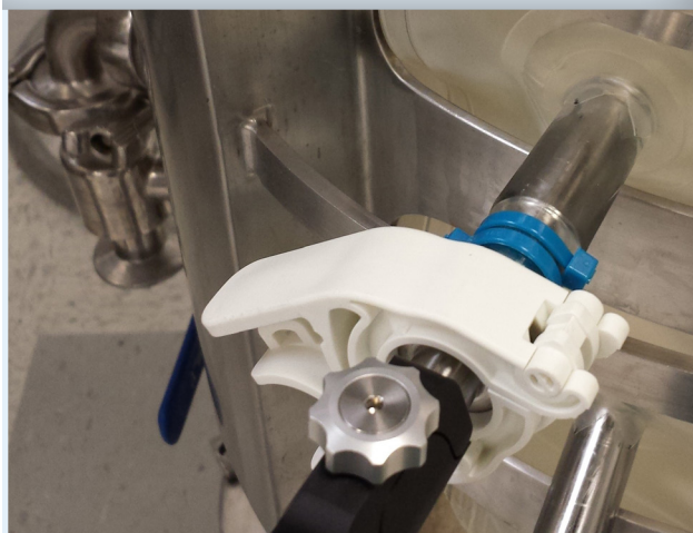
FIGURE 3: Endress+Hauser's Raman optic system for single use.
