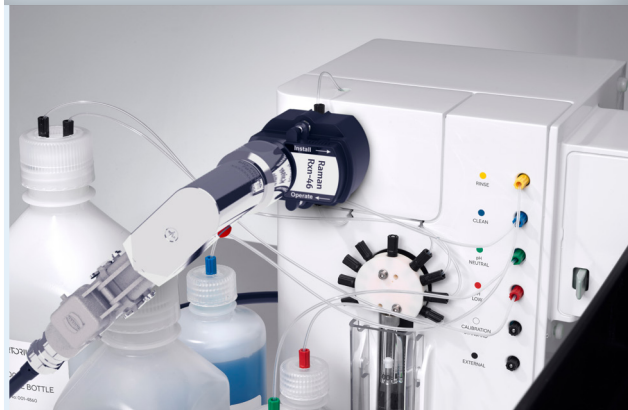
FIGURE 2: Endress+Hauser's Raman Rxn-46 bioprocess probe integrated with the Ambr® system from Sartorius.
