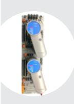
Servo Valve Positioner Module (SVPM) providing fast performance for closed-loop valve positioning.
