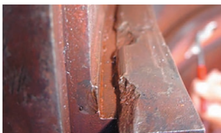
Figure 4: Severe fretting wear in casing T-slot groove
