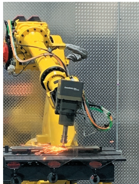
This Fanuc CNC machine at the Siemens Innovation Center is grinding a part
