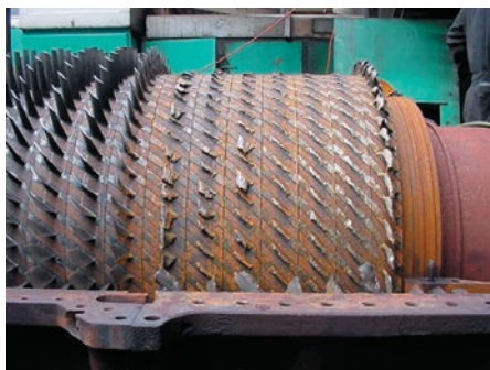
Figure 6: Catastrophic compressor failure from casing hook fit failure and vane liberation
