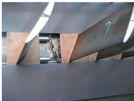
Figure 7. Stator vanes & shim assembled with dowel spring pins into a ring segment configuration within the compressor casing
