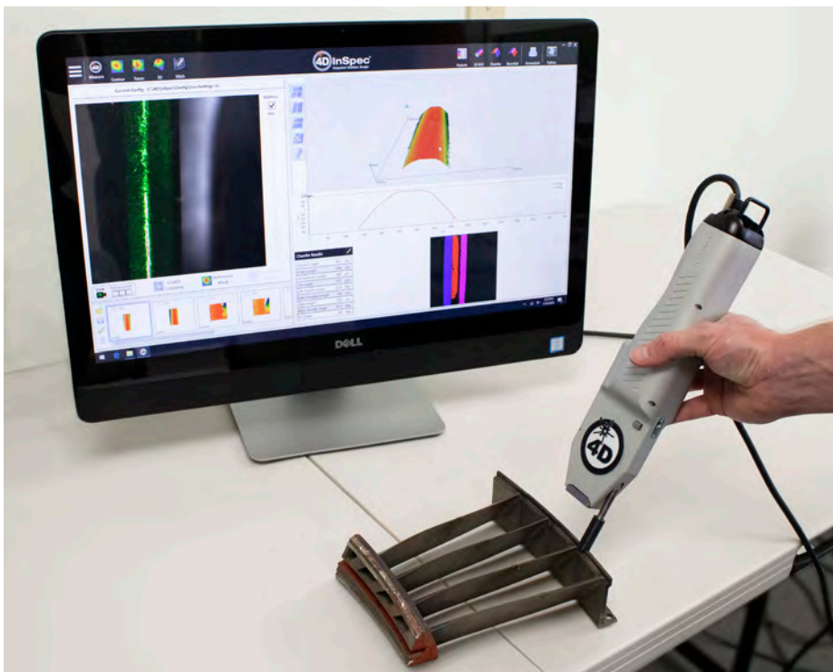
The analysis program on this handheld edge-break gauge, known as 4D InSpec, detects and calculates radius of curvature of an edge break on this turbine blade part. Courtesy of 4D Technology Corp.
