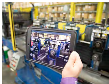
Plant operator using Regal Beloit controls to interact with a condition monitoring system using augmented reality
