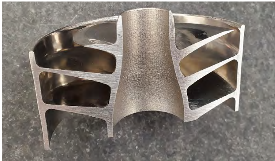
Cross-section of a CO 2 pump inducer produced using 3D metal printing by Velo3D. Photo credit: Barber-Nichols
