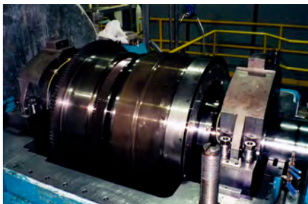
Size 220 SSS Clutch installed in 30 MW peak load steam turbine generator plant with Rolls Royce Avon gas turbines in 1971 in Sweden continues to provide synchronous condensing; reactive power, spinning reserve and grid inertia.
