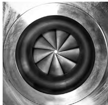
IGV blades at the inlet of a compressor pre-swirl gas flow entering the impeller, reducing the amount of work needed from the main driver.
