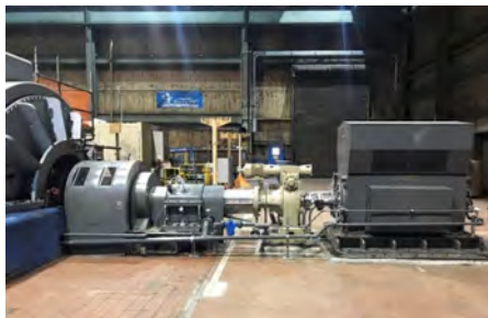
5,000 HP acceleration unit designed and built by EME Corp. using a Koenig Engineering starting & turning gear module with duo-concentric SSS turning gear and starting clutches installed to automatically connect/disconnect the acceleration system to the generator
