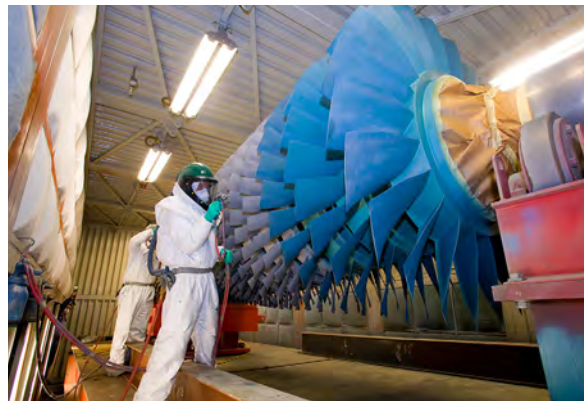
Extensive preparation is required to ensure specialized coatings bond properly with substrate materials.
