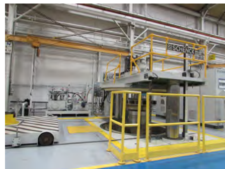
Figure 2: The overspeed test pit. The mandrel assembly is positioned on the cart (far left), which is rolled under the overspeed machine where it is fastened to the spindle. It is lowered into the pit, and a vacuum pump evacuates the chamber to minimize the power required to drive the impeller and heat generation associated with windage.
