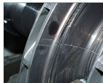
Figure 1: Sulfide-stress-cracked impeller from a plant where the operator failed to specify hydrogen sulfide in the gas.
