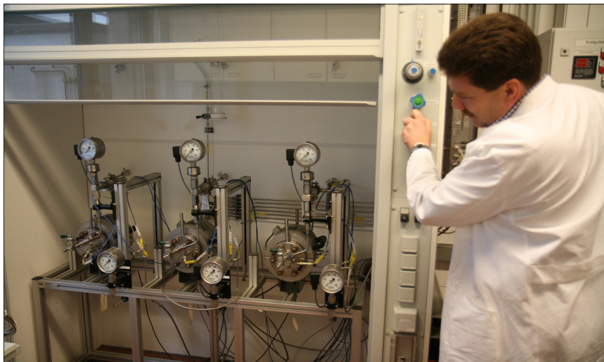
Figure 3: Siemens Energy proposes a test method where corrosion-resistant autoclaves are required to perform the tests on pre-stressed specimens at elevated pressures and temperatures.
