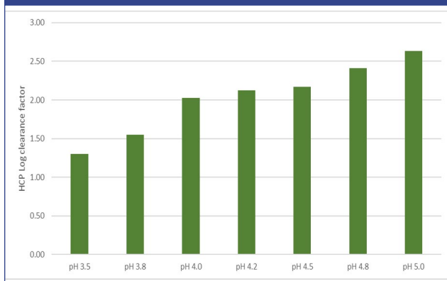
FIGURE 3: Log reduction of host cell protein levels associated with mAb X after protein capture using Praesto Jetted A50 HipH with elution buffer pH from 3.5 to 5.0.
